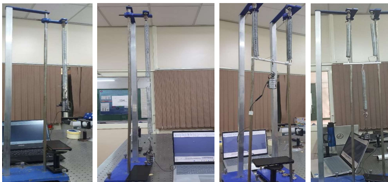
Figure 3: Experimental setup for: a. single spring, b. series configuration, c. parallel configuration, d. parallel-series configuration
