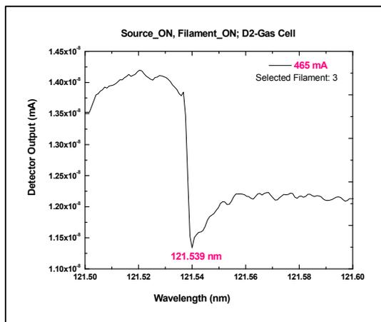
Fig. 4: Registered photo-absorption event in D2-gas cell
