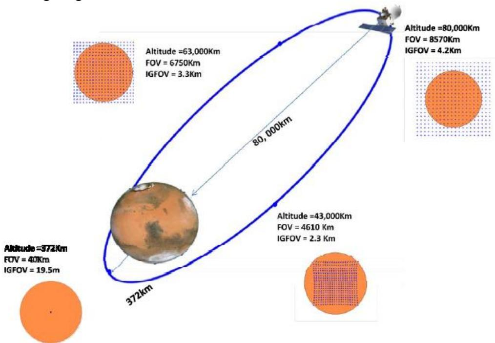
**Fig.1: Coverage with MCC from different orbital heights**
