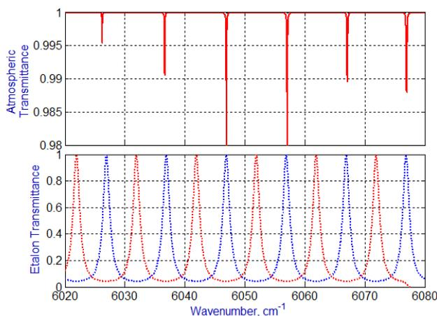
FIG.4: Spectral transmittance of FPEs of methane (blue dotted line) and reference channels (red dotted line) simulated based on design parameters. Red solid curve give atmospheric transmittance due to  $\text{CH}_4$  absorption.
