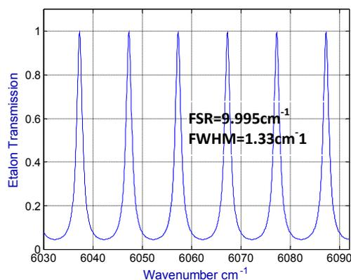
FIG-1B: Transmittance of FPE filter estimated for the design parameters  $d=0.03\text{cm}$ ,  $n=1.44$  and  $R=0.85$
