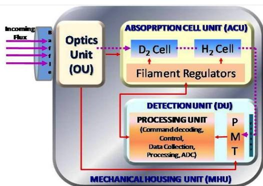
FIG. 2: A cartoon of LAP instrument configuration
