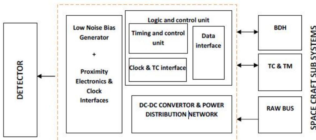
**Fig.6: Block Diagram of Camera Electronics**
