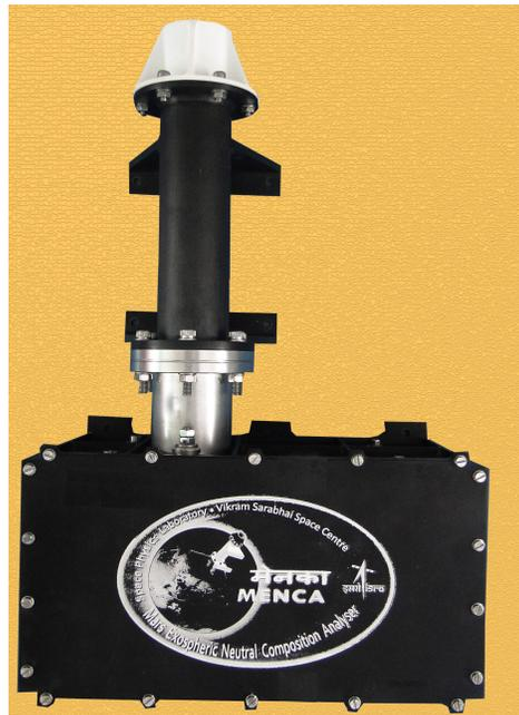
Figure 2: MENCA experiment aboard the Mars Orbiter Mission of India.
