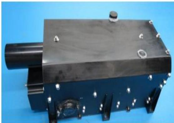
FIG. 1: LAP instrument flown in MOM spacecraft
