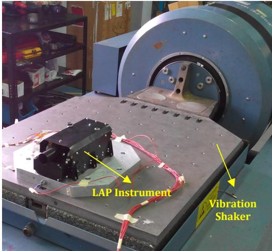
Fig. 6: LAP instrument on Vibration Shaker during it Qualification
