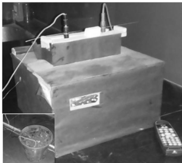
Fig. 2: Electric arc generation set up using electronic waste.
