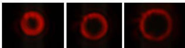
Figure 8: Experimental Intensity distribution of an optical vortex with topological charge (a)  $l=1$ ; (b)  $l=2$ ; (c)  $l=3$ .
