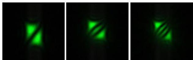
Figure 9: Intensity distribution of optical vortices of order 1, 2, and 3 after passing through a tilted plano convex lens with solid state laser at 532 nm.
