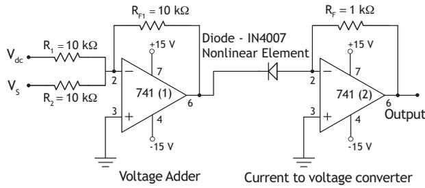
Figure 2: A diagram of a circuit designed to study the nonlinearity of a *PN*-junction diode. Two 741 general purpose operational amplifiers with a *PN*-Junction diode IN4007 are used in the circuit. Output of an inverting voltage adder is applied across a *PN*-junction diode. The output voltage of the circuit is proportional to current passing through the *PN*-junction diode.
