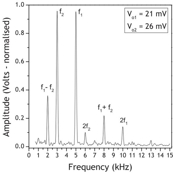
Figure 6: A frequency spectrum of the output voltage waveform shows the sum ( $f_1 + f_2$ ) and difference ( $f_1 - f_2$ ) frequency generation. Second harmonics of frequencies  $2f_1$  and  $2f_2$  corresponding to each input voltage waveform are also produced.
