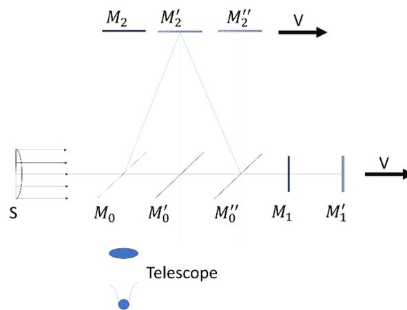
Figure 1. Line sketch of the arrangement for the Michelson – Morley experiment.
