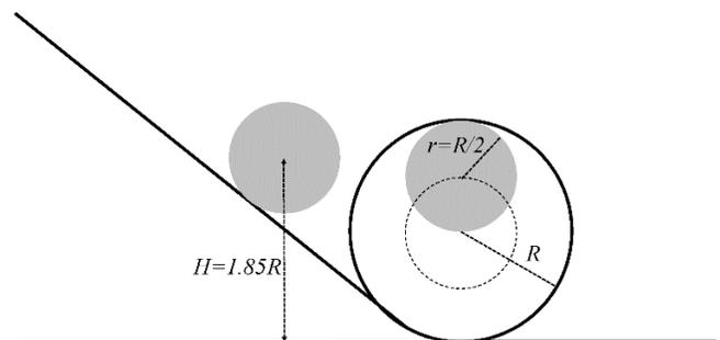
Fig. 3. The initial position and the position of the ball at the highest point for  $2r=R$ . Dashed line is a trajectory of the center of mass.
