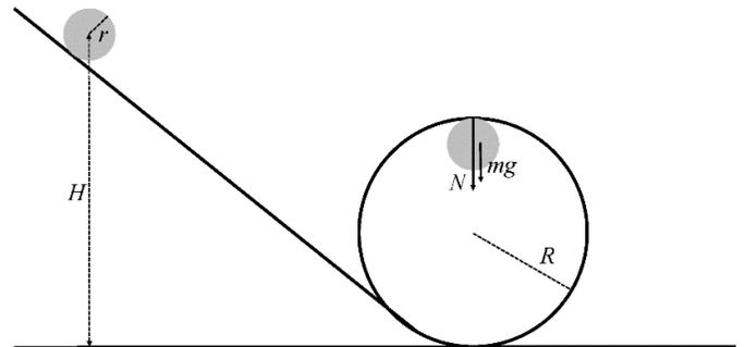
Fig. 1 Solid sphere on a loop-the-loop.
