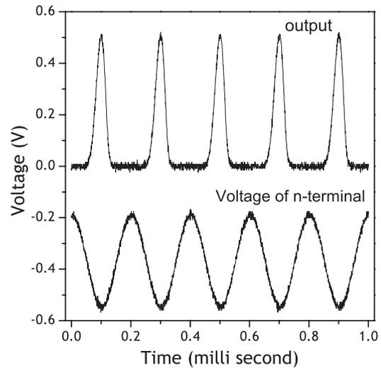
Figure 3: A plot showing an applied sinusoidal voltage across a *PN*-junction diode (lower plot). Output voltage  $V_t$  (upper plot) is linearly proportional to current passing through the diode. It is clearly shown that a sinusoidal input voltage gives rise to a non-sinusoidal output voltage due to the intrinsic nonlinearity of the diode.
