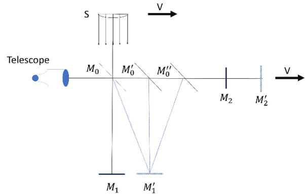
Figure 2. Set up for the Michelson – Morley experiment after being rotated through  $90^\circ$ .
