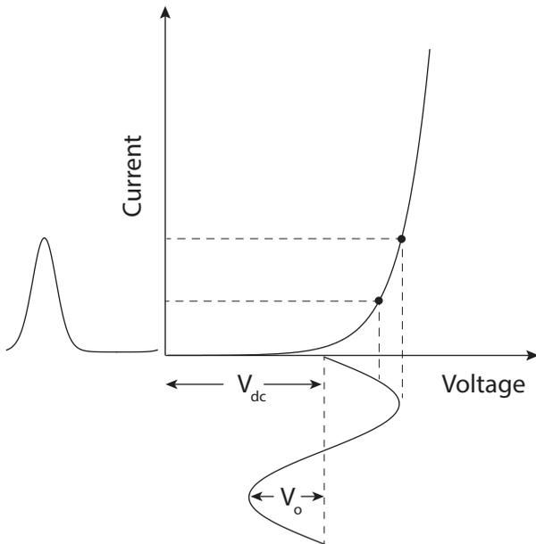
Figure 1: A schematic showing an exponential dependence of current on the forward bias voltage across a *PN*-junction diode. A variation of diode current for a sinusoidal bias voltage of amplitude  $V_o$  with a dc offset  $V_{dc}$  is also shown.
