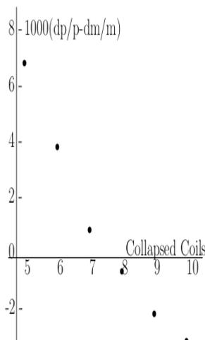
Figure 3. Sign change of  $(dp/p - dm/m)$  occurs between coils 7 and 8 at maximum speed.
