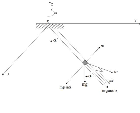
Figure 5: Forces acting on the bead as observed by an observer in the Inertial frame.
