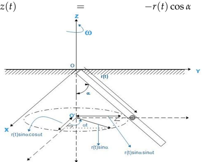
Figure 4: Orientation of the rod in cartesian coordinates.  $r(t)$  is the instantaneous position vector of the bead from the pivot
