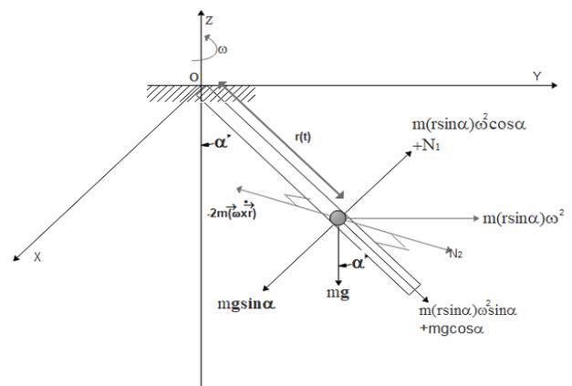
Figure 2: Forces acting on the bead as viewed by an observer in the Non- Inertial Frame
