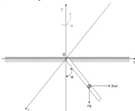
Figure 1: Bead sliding along a rotating rigid
