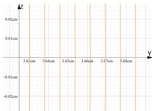
Figure 9: Circular fringes as appear within small field of view.
